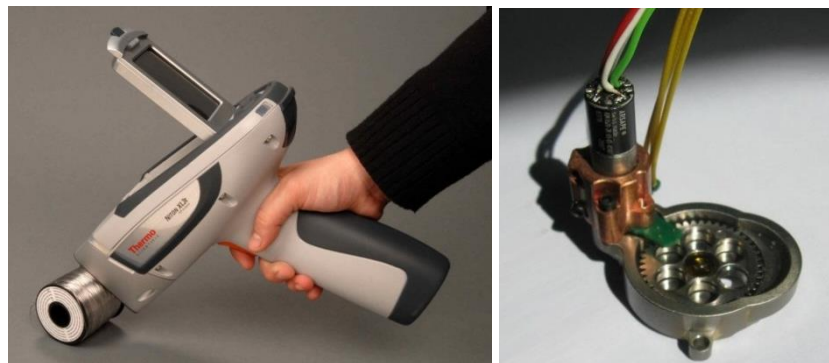
Figure 15 : Hand-held X-ray analyzer (left) and an example of filter wheel integrating a stepper motor (right).
