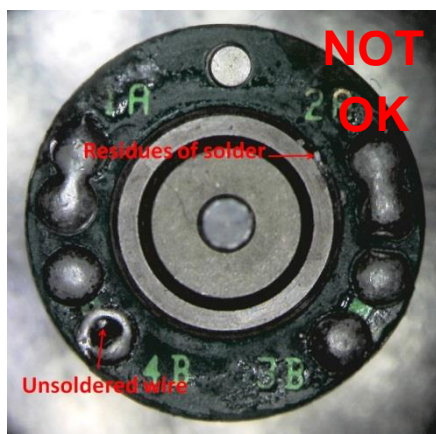
Figure 4 : Good and bad examples of a solder on various stepper motors.
